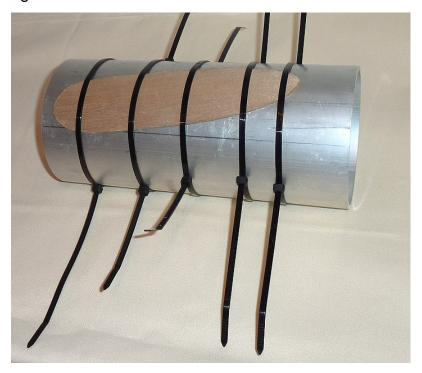
Baked in the oven at 150°C for about half an hour, the result is stable blades. I make the hub out of glued tissue tubes wrapped round a 1.6mm drill. I can then play with the pitch to get an intuitive best angle.
