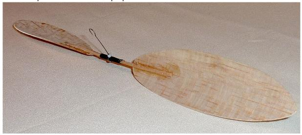
The problem is that, though twisted correctly, the blades are fairly flat so are not efficient. I need built-up blades, with an aerofoil section covered with film, that will turn more slowly. I can then use more of the turns and hopefully use longer and probably thinner motors.
