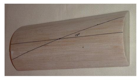
My propellors will not be as flimsy as the ones for FAI models. I should be able to build the outline around a template on the curved building board then remove the template and add the ribs. I will then glue the whole onto the propellor spar in a jig. I will also use the carving template as the starting point for marking out a sheet aluminium template for cutting the ribs.
